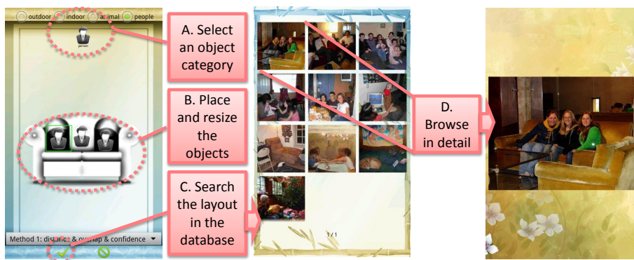
Fig. 1. Interface of the search client. The user first draws the object layout as the query, then search and browse the matched images.
