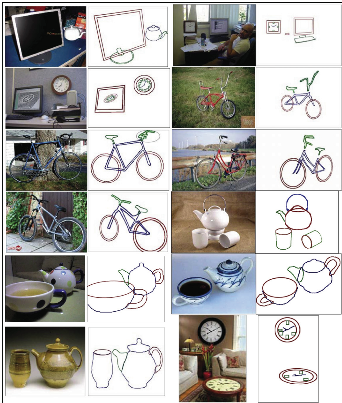
Fig. 7. Parsing/recognition results for compositional object categories, including bicycles, clocks, monitors, cups and teapots. The most informative parts detected in the bottom-up stage are denoted in red, such as the bicycle wheels, monitor frames, clock frames and cup lips. The predicted and matched parts using top-down knowledge are denoted in blue, such as the clock hands, the bicycle frame, cup handles and teapot bases. The parts with weak image evidence (noisy or occluded), which are hallucinated and matched using the prior models, are denoted in green, such as the clock numbers, monitor base, teapot spot and bicycle seat/handlebars. The wrong hallucination results, which do not match human perception, are indicated by circles [25]. (For interpretation of the references to color in this figure legend, the reader is referred to the web version of this article.)
